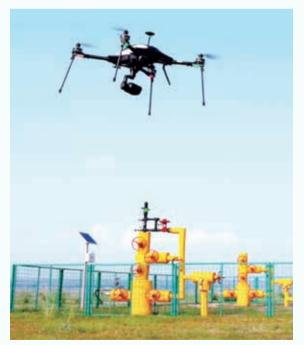
Routing inspection by drones at Changqing
